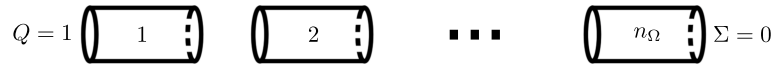
Figure 3: Serial network of n_\Omega cylinders connected by \mathcal{C} = n_\Omega - 1 couplings. On the left we impose a unitary flow rate, while on the right a no-stress Neumann boundary condition is applied.
